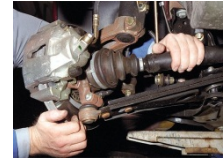
This shaft transmits drive to the wheels
