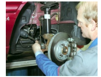
Checking for leaks
