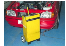
Fast charger with engine starting facility
