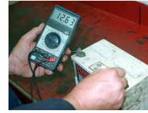
Battery voltage readings...
