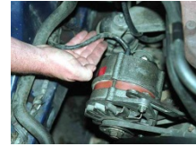
Alternator cables to battery
