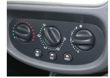
Air conditioning controls
