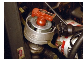
Distributor for engine speed and position sensing
