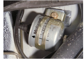
Filters are directional
