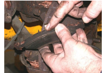
Checking the pad lining thickness
