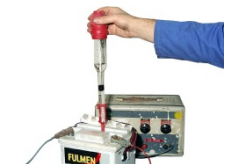
Testing a battery on charge
