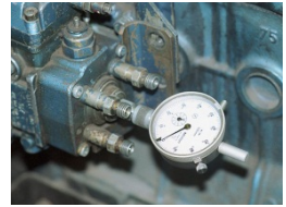
Diesel pump being timed on engine
