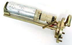
Electric fuel pump in the tank
