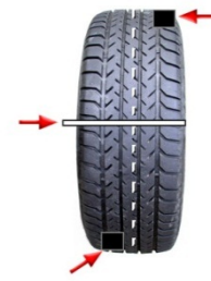
Statically balanced but dynamically imbalanced
