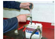
Checking batteries on charge with a hydrometer
