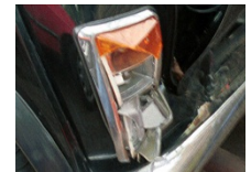
Damaged rear light lens
