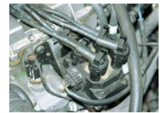
System requiring no distributor
