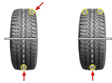
Wheels that have been statically balanced
