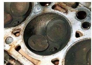
Valves in position
