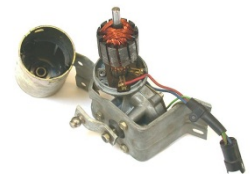
Motor brushes and armature
