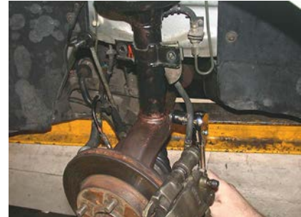
Remove the lower fixing
