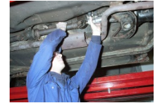
Checking the universal joints
