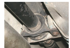
This bearing prevents propshaft whip
