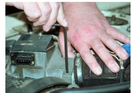
Air flow meter adjustment
