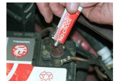
Terminals with battery grease
