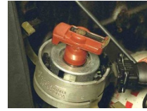
Rotor in place
