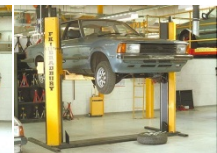
Two post lift in use
