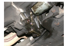
Transmission oil leak
