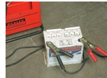
Battery caps removed during fast charging
