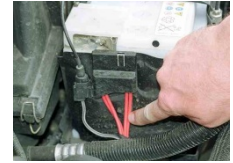
These links connect to the battery
