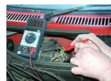
Checking voltage at the resistor pack
