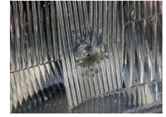
Damaged headlight lens
