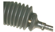
Damaged steering gaiter
