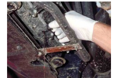
Coolant being drained
