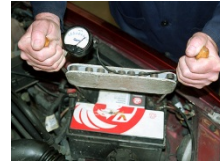
Heavy duty discharge test on the vehicle
