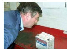
Blow away any hydrogen gas before starting the test
