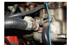
Water-heated inlet manifold
