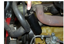
Oil separator connected to the crankcase
