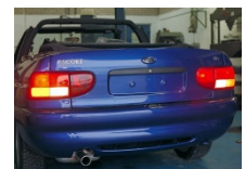
Stop and reverse lights form part of the rear light cluster
