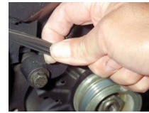
Drive belt test
