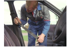
Checking the belt condition
