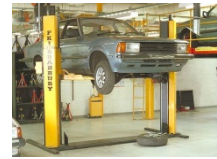
Two post lift in use
