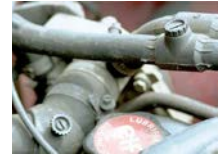
Bleed valves in cooling system
