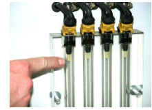
Injector flow test
