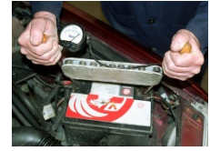
A good battery under test
