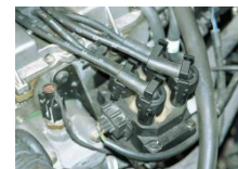
System requiring no distributor
