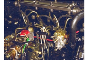
Injection pump, pipes and injectors
