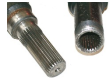
A splined joint connects to the gearbox
