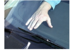
Checking for hot air
