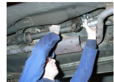
This shaft transmits drive to the final drive
