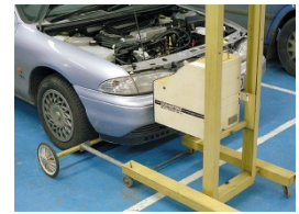
Beam setter in use
