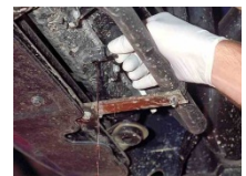
Radiator being drained
