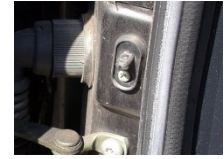
Switch positioned in the door pillar
