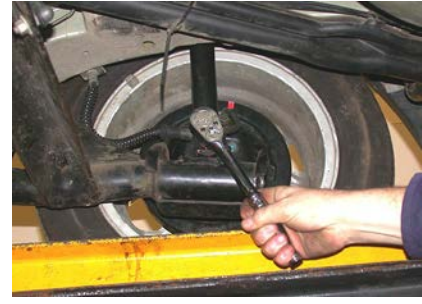
Remove the lower fixing
