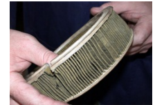
This air filter needs replacing!
