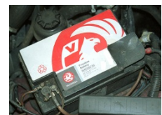
Low maintenance battery
