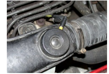
Air temperature control valve
