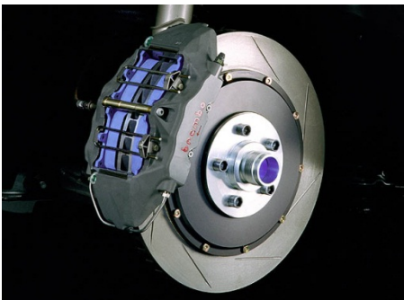
High performance pads and disc
