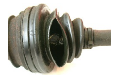
Damaged CV gaiter
