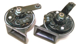
Horns removed from vehicle
