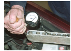
For most car batteries the voltage should hold at 9 or 10 V for 9 or 10 seconds
