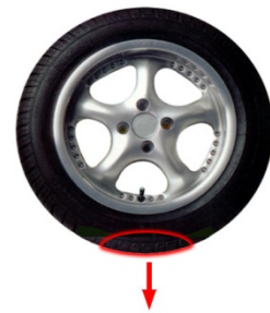
Wheel with an out of balance mass
