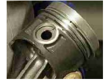
Pin in place
