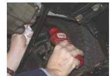
Filling the gearbox oil
