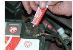
Clean and apply battery grease
