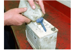
Open cell battery - with removable caps
