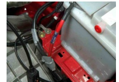
Checking battery carrier
