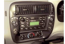
Fresh air fascia vents
