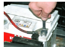
Undoing the battery terminal
