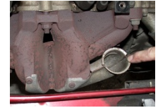
Pick-up for hot air on an exhaust manifold
