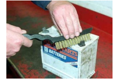
Cleaning the battery terminals
