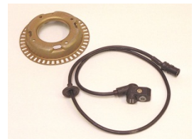
Inductive speed sensor
