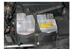
Battery security clamps
