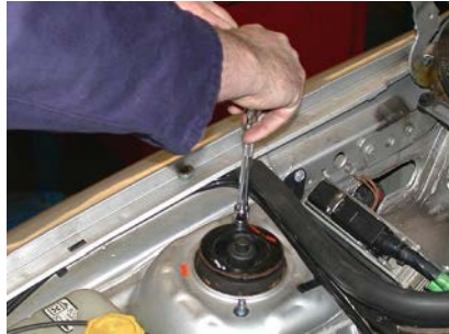
This damper is part of the strut
